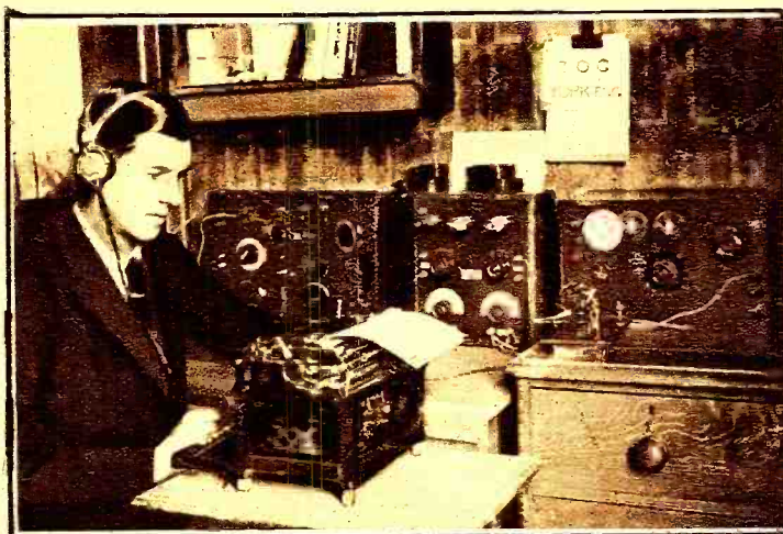
In Spite of the Restrictions on English Amateurs, Mr. Cooper has Succeeded in Designing and Constructing a Very Efficient Station. With Duo-Lateral Coils and High-Frequency Amplification He Copies Long Distances. The Transmitter Output is Limited to 10 Watts, but 50 Miles is Covered Consistently.
